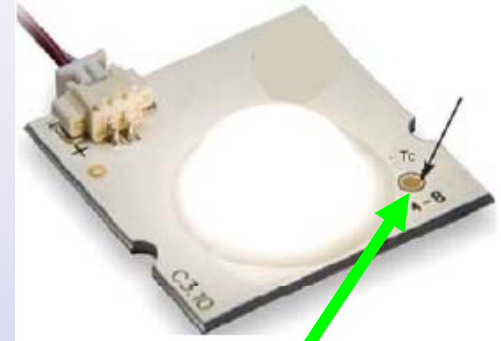
Designated Temperature Test Point
