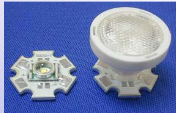
Secondary optic - 10 to 15% losses of flux
