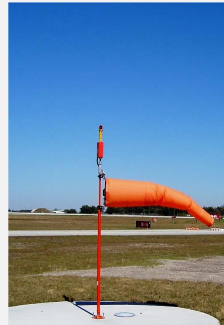
Uncertified Internally Lighted L-806 8' Supplemental Wind Cone
