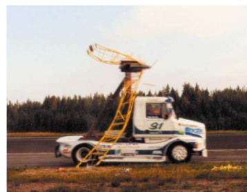
Fig. 5 Finnish design concept built up from small diameter fibreglass/epoxy tubes [6, 9]
