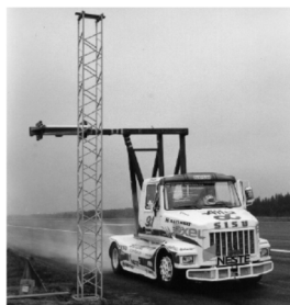
Fig. 5 Finnish design concept built up from small diameter fibreglass/epoxy tubes [6, 9]
