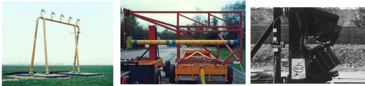
Fig. 6 Dutch design concept built up from large diameter fibreglass/epoxy tubes, test configuration and wing impactor [7]
