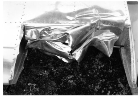
Fig. 11 Typical impact damage on the standard wing impactor
