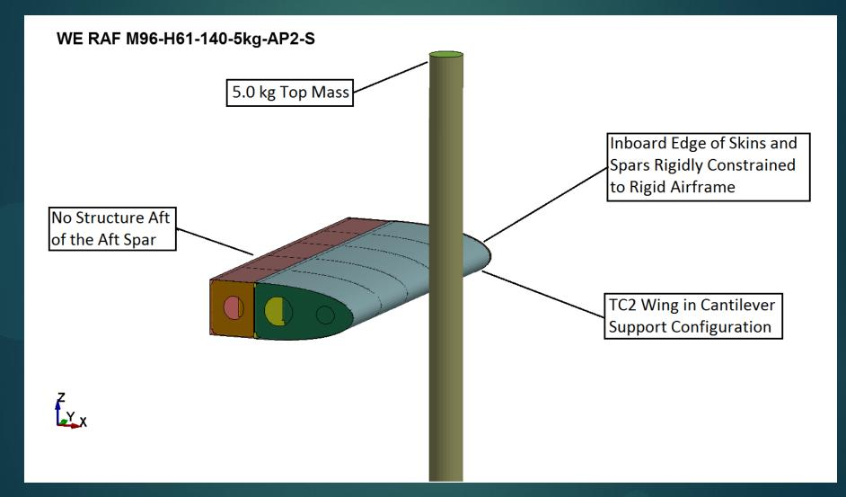
Impact Test Simulation: Aluminum Pipe 2 mm wall – 5.0 kg Top Mass
