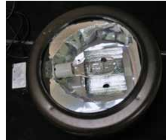
HID Fixture with Single Light Source and Reflectors
