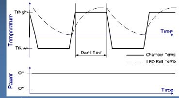
**IEC 60068-2-14** : Test the ability to withstand rapid changes of ambient temperature."
