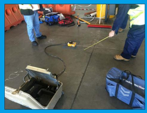
Concrete Scanning Equipment for Locating Existing Utilities and Rebar
