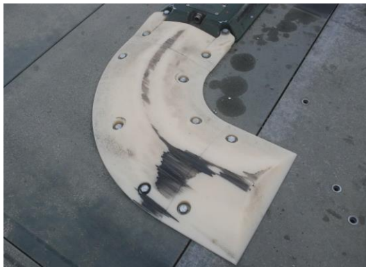
AM2 Mat concept – ABS plastic after 25 “hits” from M31 tape sweep connector
