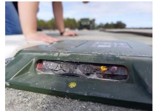
Damage from Tape Connector
